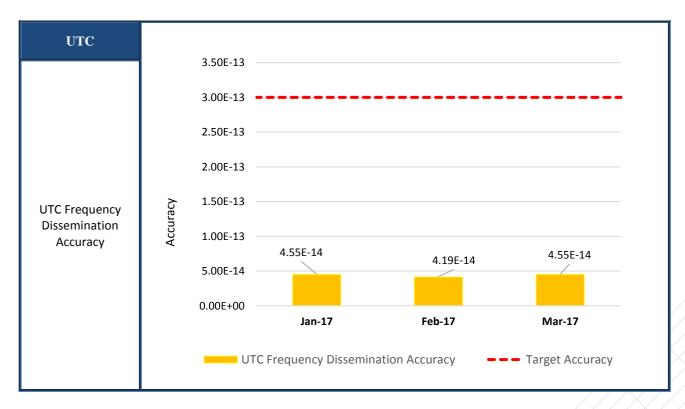
Figure 9: Long-term 95<sup>th</sup> percentile of UTC Frequency Dissemination Accuracy
