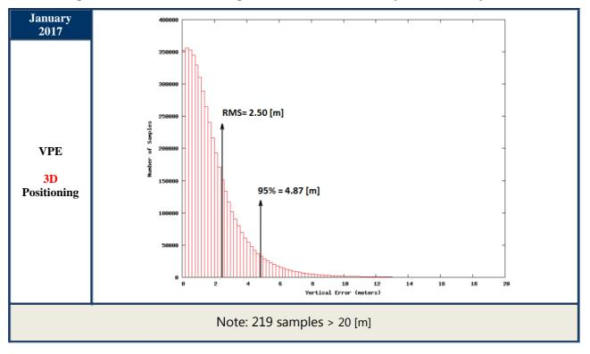
Figures 16: Vertical Positioning Error (VPE) for Galileo only users (February 2017)
