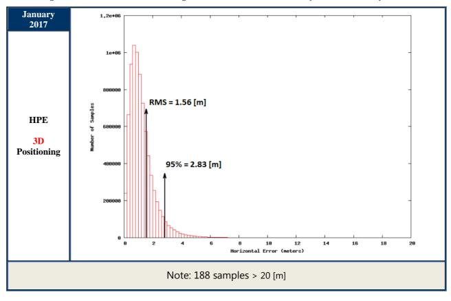
Figure 12: Horizontal Positioning Error (HPE) for "Galileo-only" users (January 2017)
