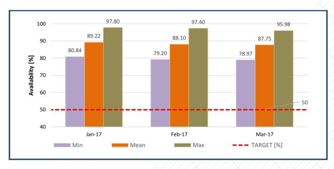
Figure 11: Availability of the Galileo Horizontal Positioning Service with Accuracy ≤ 10 [m]
