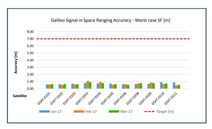
Figure 4: Monthly Galileo SIS Ranging Accuracy (95<sup>th</sup> percentile) "for any satellite", measured during reporting period for worst-case, Single-Frequency (SF)
