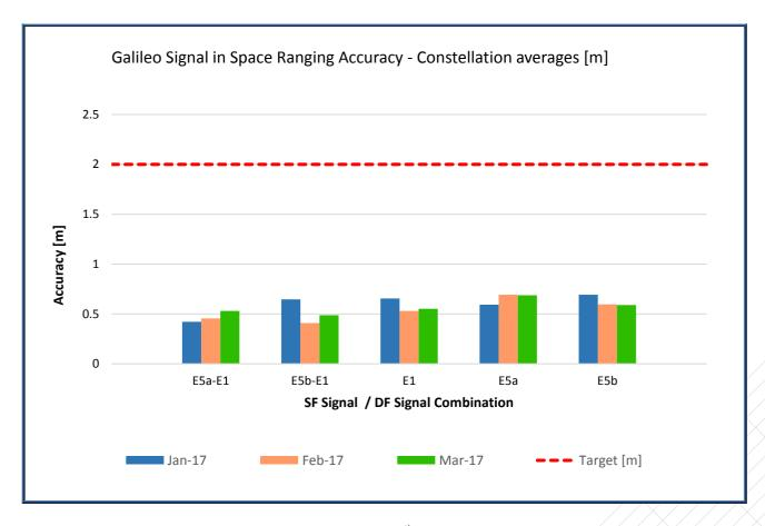
Figure 5: Monthly Galileo SIS Ranging Accuracy (95<sup>th</sup> percentile) "over all satellites" (constellation average), measured during the reporting period
