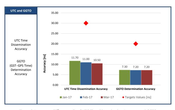
Figure 8: Long-term 95<sup>th</sup> percentile of UTC Time Dissemination Accuracy and GGTO Determination Accuracy
