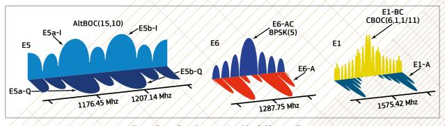
Figure 3. Signals transmitted by Galileo satellites
