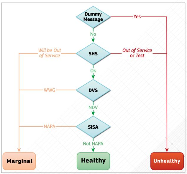
Figure 4. Example of a Decision Tree for the Determination of the Status of broadcast SIS.
