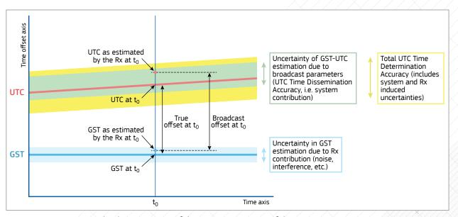
Figure 5. Graphical representation of the various components of the UTC Time Determination Accuracy.
