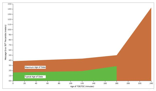
Figure 7. Typical SISE vs. Prediction Time from ToE (All Batches)<sup>17</sup>
