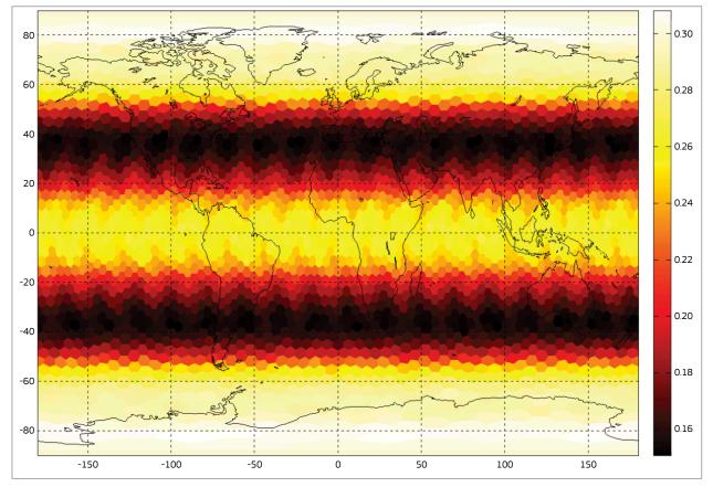
Figure 8. Availability of PDOP (colour coded) for the constellation of 9 satellites, considering PDOP  $\leq 6$ .
